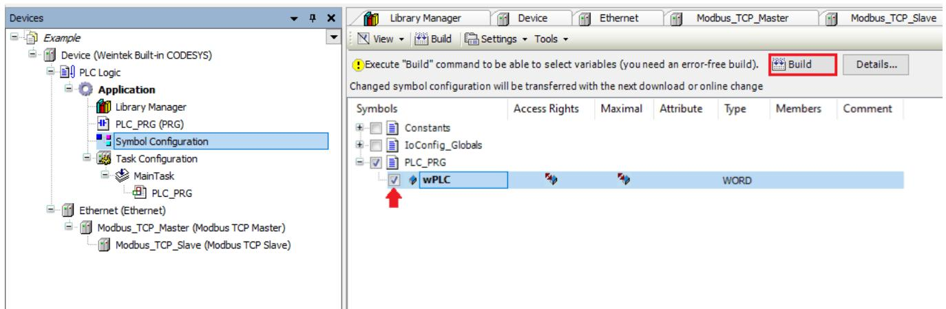
Step 22: Within the “Build” tab, click on “Generate code” and an .xml file called “[PROJECT NAME].Device.Application.xml” will be saved within the same folder as the project file. We will use this file to import tags into EasyBuilder Pro.
