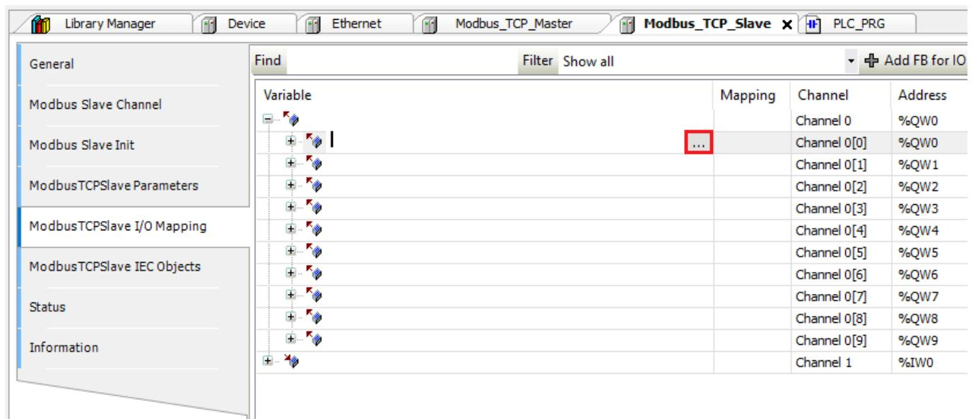
Step 19: Ensure that the desired project variable is selected and click “OK” to map this variable to the I/O point:
