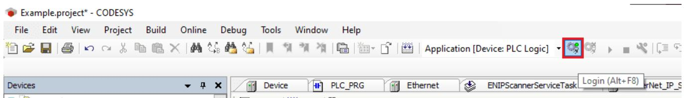
Step 24: Click the “Start” button to place the Codesys application in “RUN” mode.
